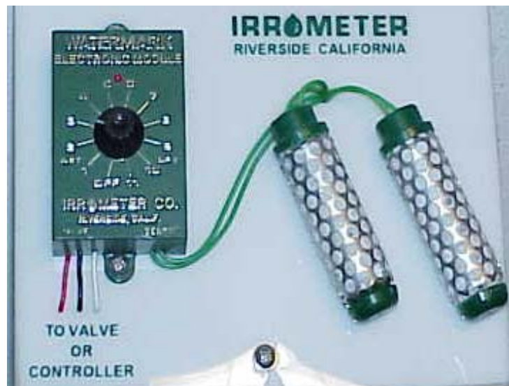
Picture is shown for an example of a soil moisture sensor. Several styles and brands are available and no endorsement of any manufacturer is intended.
