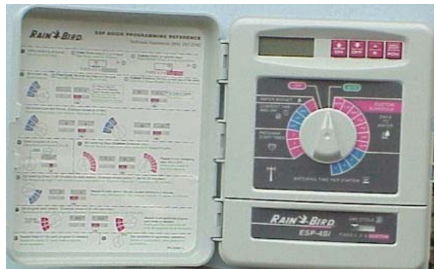
Automatic Irrigation Controller
