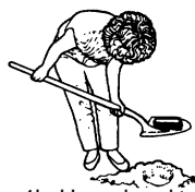
Figure 1b. Use a hand trowel, shovel or other garden tool. Trim out soil of uniform thickness to the recommended depth.
