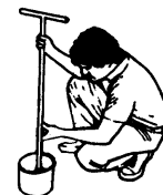
Figure 2. Place 10 to 15 soil cores into a plastic bucket; mix, dry, and transfer to a bag.
